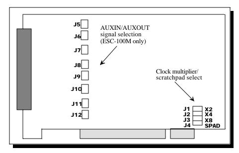
Figure 5 --- Jumper/connector locations
